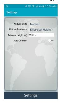
**Warning:** Do not enter the antenna height both in Eos Tools Pro and Collector. It is preferable to leave this field blank in Eos Tools and enter the antenna height in Collector.
