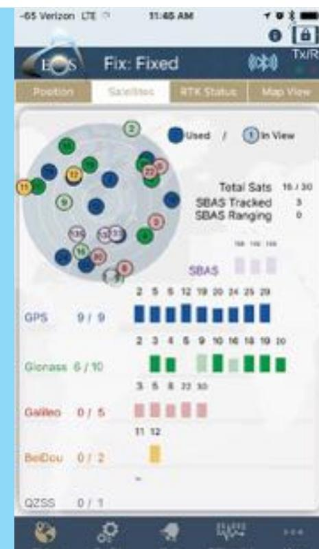
↑ The GIS team also used the Arrow Gold GNSS receiver from Eos Positioning Systems to monitor position accuracy in real time.
