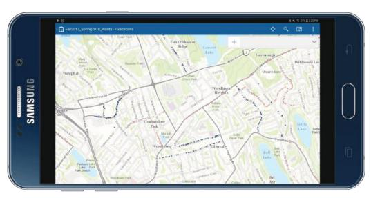
Interns mapped urban trees in real-time with submeter accuracy using Samsung tablets, Esri's Collector for ArcGIS app, and Arrow 100 GPS (GNSS) receivers.
