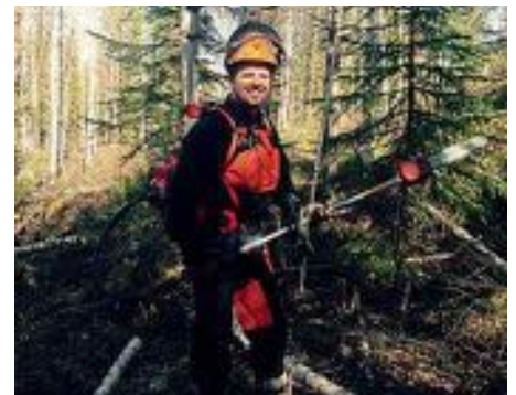
Clearing the boundary with a special saw – a hybrid between a brush cutter and a pole saw
