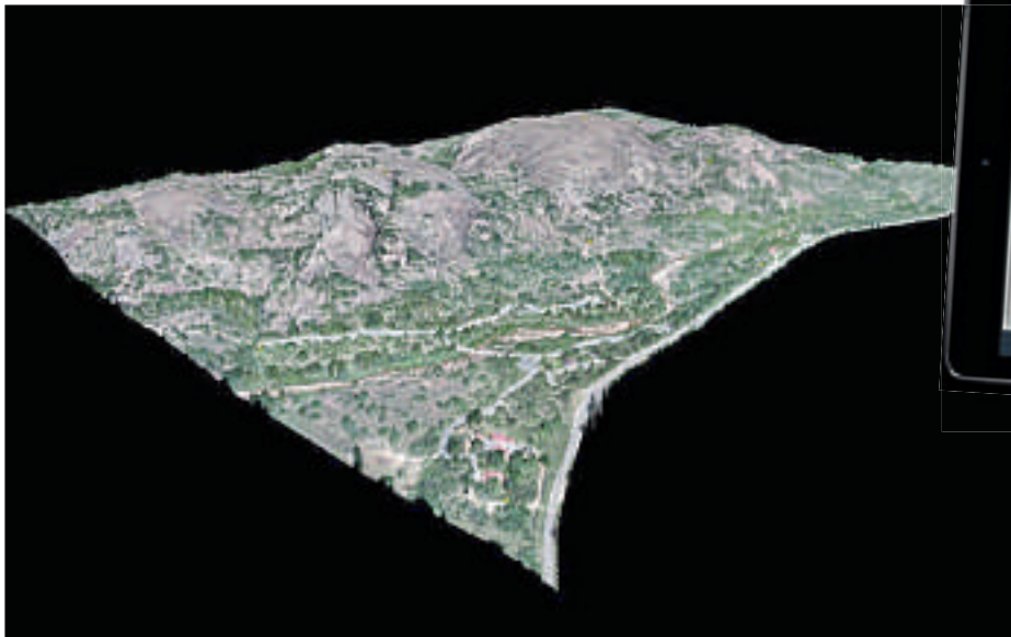
RAS delivered a complete, survey-grade orthophoto mosaic to the park rangers and university educators. They also provided a digital surface-elevation map with three contour levels (1.5m, 3m, 6m) and a 3D model
