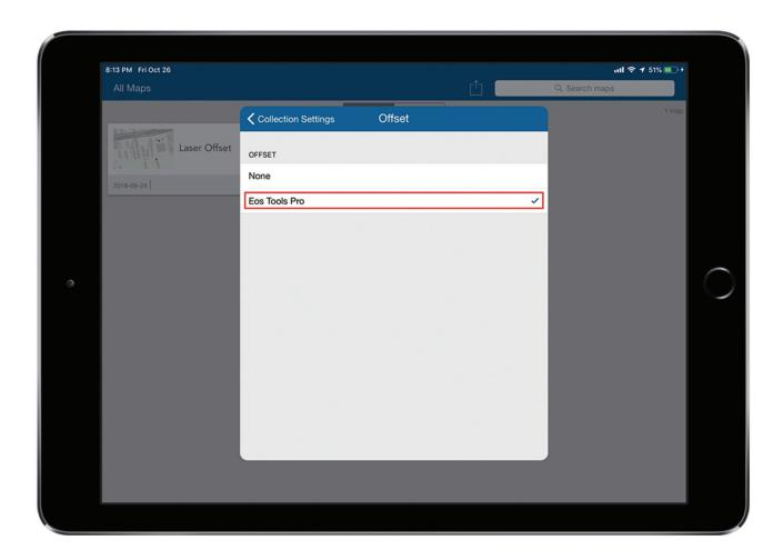
Next, let's make sure Eos Tools Pro is set up to provide Collector with orthometric heights.
