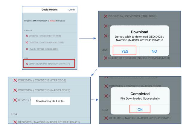
c) Once the files are downloaded, a green checkmark  $\sqrt{}$  will replace the X on the left of the listed Geoid model. This confirms that all the geoid model files are available locally on your device. Make sure to tap on the Geoid model to select it (a blue checkmark  $\sqrt{}$  will be displayed on the right to confirm the selection).
