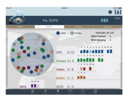
You can see in the upper right corner of the screen that **24 satellites**, out of 33 in view, are being used. That's a huge leap from even a couple of years ago. Let's break down where the 24 are coming from:
