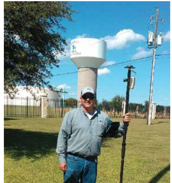
Benjamin Rucks stands outside the Rockett SUD office with one of the utility's water towers in the background. He is holding his mobile GIS solution for field data collection, using ArcGIS® Field Maps, an Eos Arrow Gold® RTK receiver, and an iPad®.
