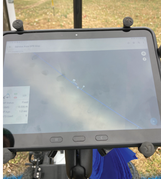
Left: Warren County Water District Serviceman Brandon Edwards maps subsurface water mains. Middle: To detect an asset's location, he uses GPR. Right: To map it, he uses ArcGIS Field Maps on Android and an Arrow Gold GNSS receiver connected to the free the KYCORS network.
