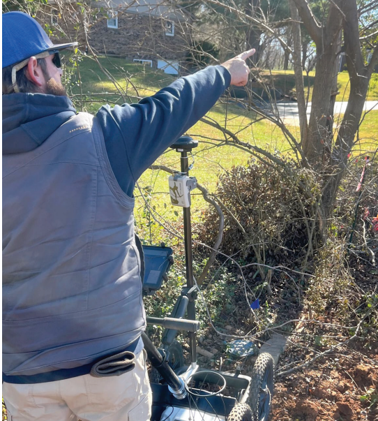
Left: Warren County Water District Serviceman Brandon Edwards maps subsurface water mains. Middle: To detect an asset's location, he uses GPR. Right: To map it, he uses ArcGIS Field Maps on Android and an Arrow Gold GNSS receiver connected to the free the KYCORS network.
