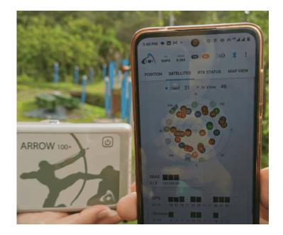
With the Arrow 100+ submeter GNSS receiver and ArcGIS Survey132, Coopeguanacaste achieved significant improvements in location accuracy. Using these technologies they accurately mapped over 52,000 electric and telecommunications poles."
