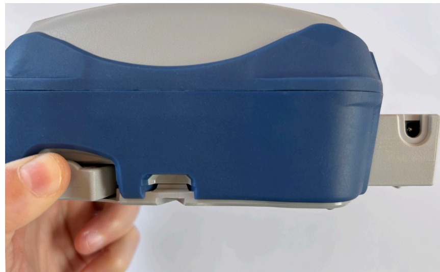
Push the two battery release latches on both sides of your Skadi GNSS receiver and pull to release the battery pack.
