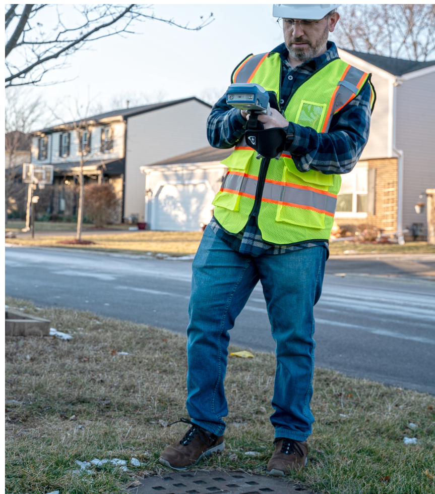
Invisible Range Pole mode is designed to continuously measure the X, Y, and Z position of the location of the ground or asset directly below the receiver.
