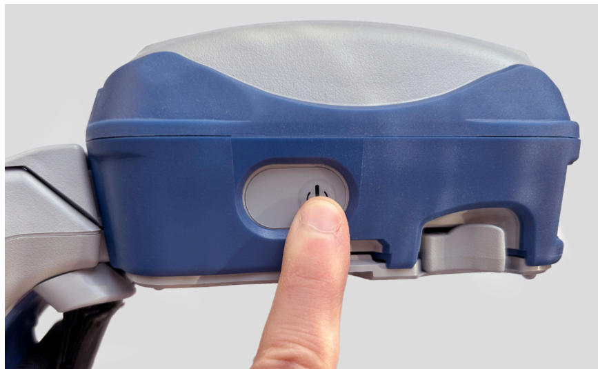
Triple-press the power button on your Skadi GNSS receiver.
