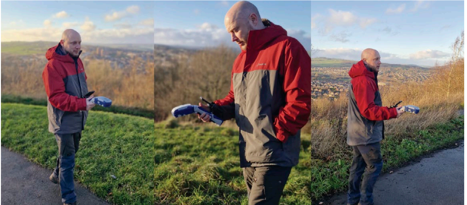
Sheffield City Council Senior Engineer Gavin Brooksbank maps a public right of way (PRoW) by using a Skadi 100 GNSS receiver for accuracy and ArcGIS QuickCapture for real-time data collection. The improved information helps justify maintenance and investments.
