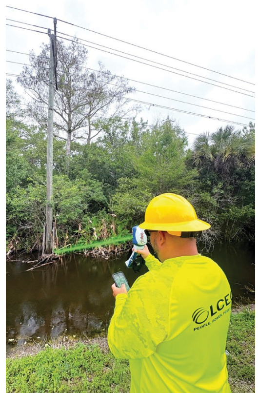
Otero uses the Skadi Smart Handle to GPS assets located across a canal like this one.
