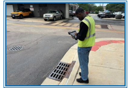
Public Works Engineering intern Kyan Muhammed maps a stormwater drain with the Arrow Gold+ in a handheld configuration, ArcGIS Field Maps, and RTK corrections.
